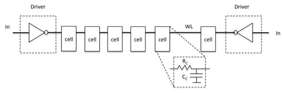
Driving from both sides reduces the "effective distributed length" of the memory array by a factor of 2. In a distributed system this effectively reduces the delay by a factor of 4. The overall delay is now:
