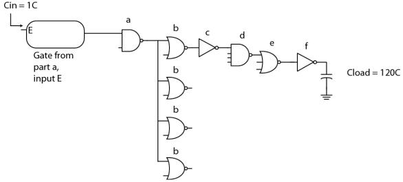
d) (4 pts) Using the gate from part a) as well as other standard logic gates, what is the path effort of the following chain of gates? All gates are also implemented in this same technology with  $R_P = \frac{1}{3} * R_N$ .
