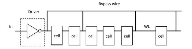
The longest connection now would be 3 \* 64 cells over the bypass wire + 32 memory cells. This translates into a delay: 0.38 \* (192 \* (Rc/10) \* 192 \* Cc) + (32 \* Rc) \* 32 \* Cc) = 0.018 nsec
